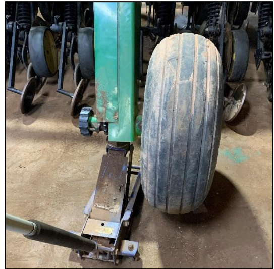
Figure 1. Hydraulic floor jack used to elevate the drive wheel.
